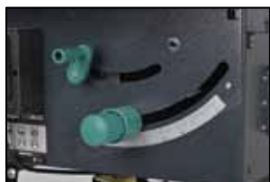
ANGLE AND HEIGHT OF SAW ADJUSTMENT
