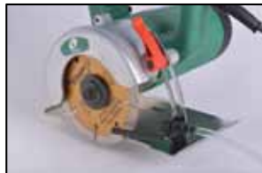
CUTTING DEPTH ADJUSTMENT
