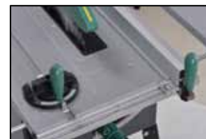
ANGLE CUTTING ADJUSTMENT
