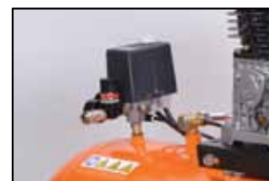
PRESSURE SWITCH, OUTPUT
