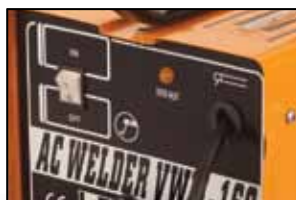
CONTROL LAMP, ON/OFF SWITCH
