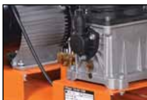
OIL LEVEL CHECK, BELT DRIVE
